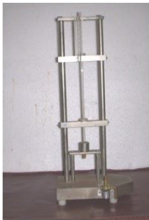
Figure2. Viscometer and plastic blood test tubes for experimentation
