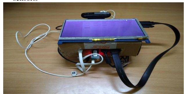
Fig 3. Final Prototype device, note that the screen is only for visualization of the workflow, the visually impaired user is going to use the earphones and have a normal conversation pertaining to the task sheet.
