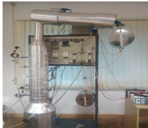
Fig.1 Real time binary distillation column
