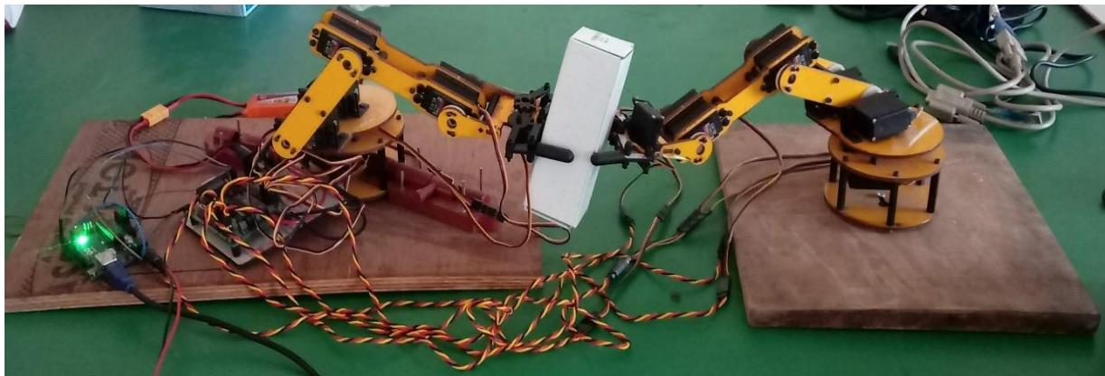
Figure 15 Sample Experimental Setup of Dual arm Cooperative Manipulator
