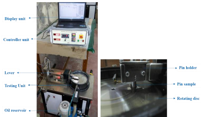
Fig.1. Schematic view of Pin on disc apparatus
