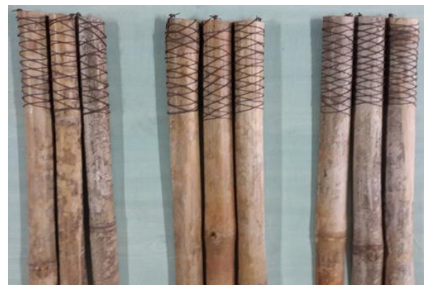
Fig. 4 Wire wrapped culms for pull out test
