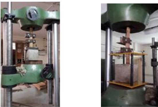
Fig. 6 Pull out testing in UTM
