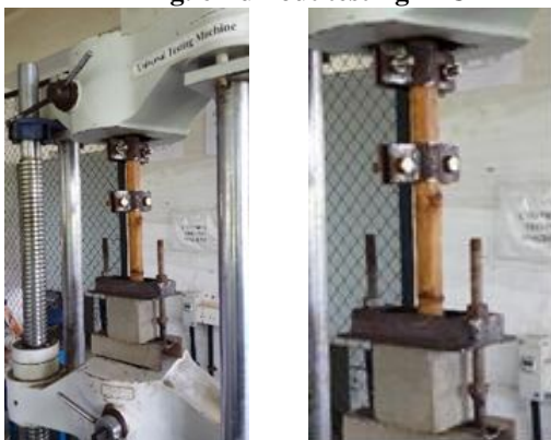
Fig. 7 Pull out testing in UTM
