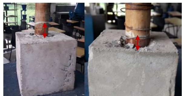
Fig. 8 Failure pattern during pull out test
