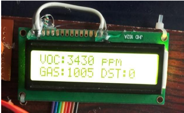
Fig 5.2.2 Exceeded level of VOC gases in air
