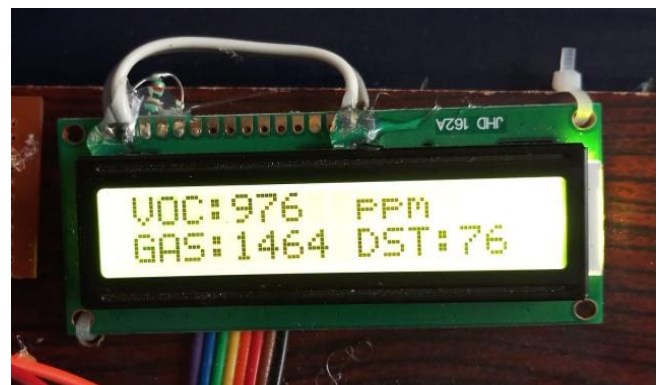
Fig 5.2.6 Exceeded level of dust and smoke in air
