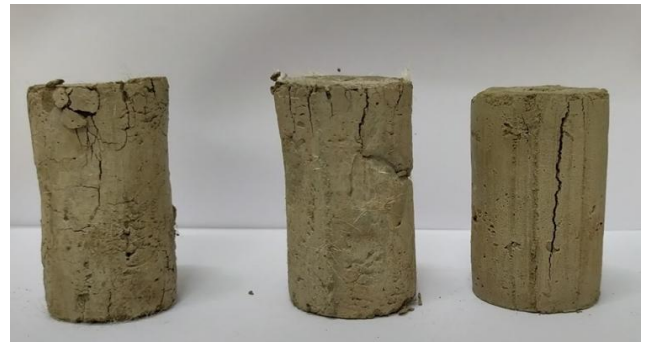
Fig. 2. UCS samples after the test.
