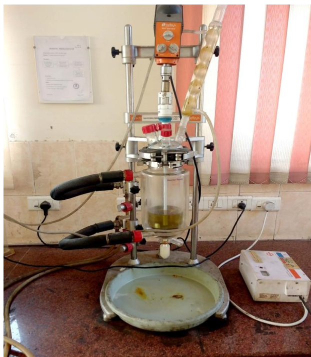
Fig. 5. Redlay reactor for transesterification
