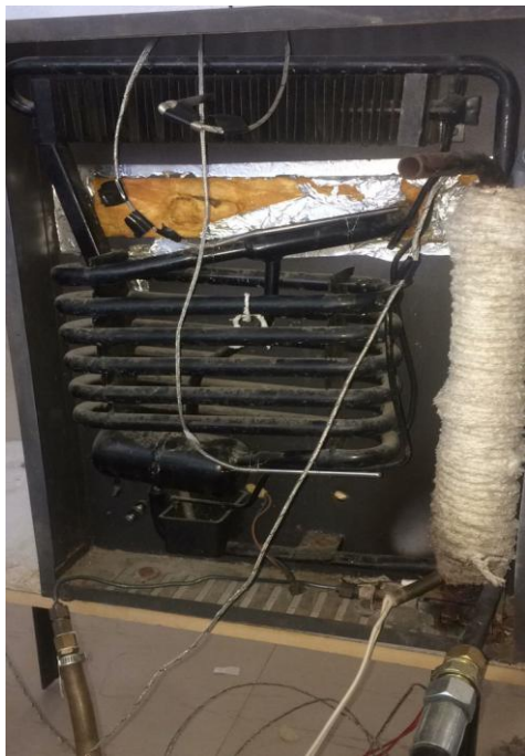
Figure 2: Fabricated Biogas Powered vapour absorption refrigeration system
