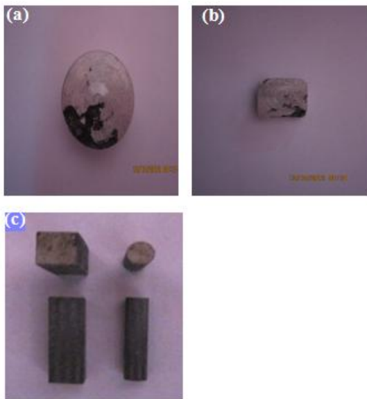
Figure 2 (a)and (b) Shows Al-Fe alloy samples turned in a lathe and (c) shows wire-cut EDM samples.
