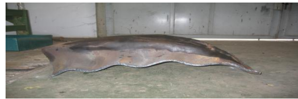
Figure 7. Fractography of a piece of a furnace at the upper fireside (side view)
