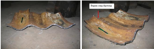
Figure 12. Fractography of the furnace - the bottom fireside that is not subjected to plastic deformation.
