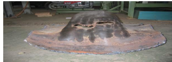
Figure 8. Fractography of a piece of a furnace at the upper fireside (front view)
