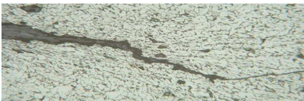
Figure 13. Microstructure in the fracture area which has a ferrite-pearlite phase. 500x
