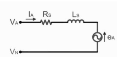
Fig.1. For Phase A PMBLDC motor Equivalent circuit
