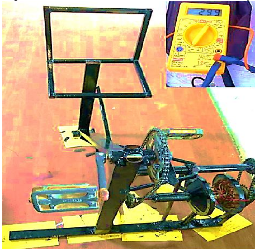
Fig. 12. Full setup of the machine consisting of parallel generator system
