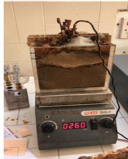
Figure 2 Experimental set up of electrocoagulation treatment in a lab-scale
