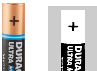
Fig. 4 Black color segmentation using L < .2 as threshold of object (right)
