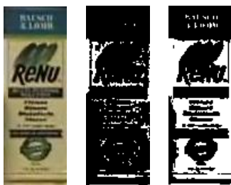
Fig. 3 White color segmentation of object(left) using L > .7 as threshold(middle) and L > .6 as threshold
