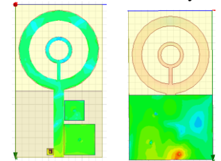
Fig 14: Current distribution in the radiating plane and ground plane at 7.4 GHz
