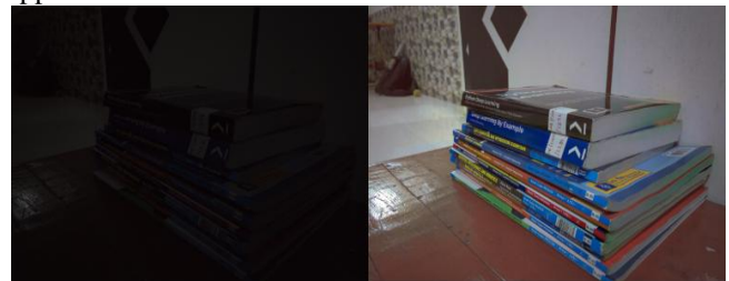
Figure 1: Image Captured in Extreme Low Light vs. Enhanced Image produced from our Convolutional Neural Network
