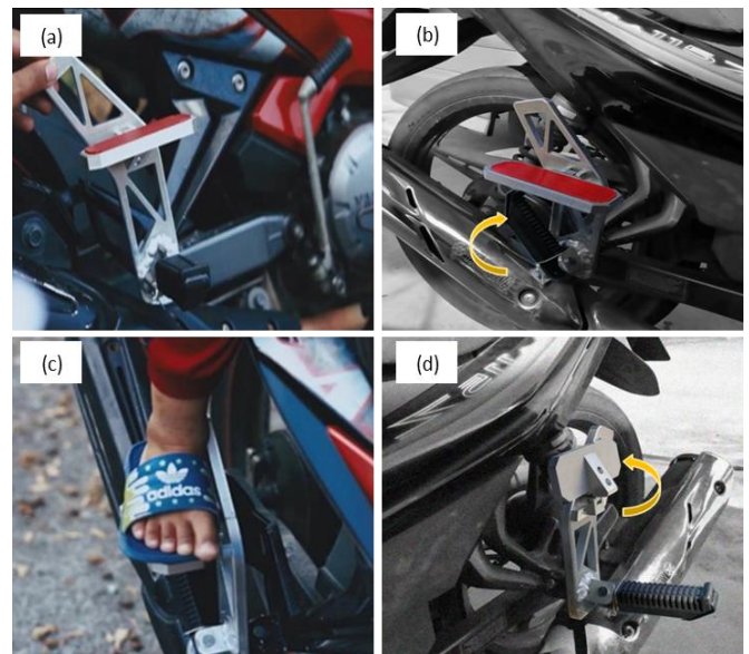
Fig. 7. (a) Installation of PIJAK foot-board (b) PIJAK foot-board being flipped down and ready to be used (c) PIJAK footboard is being used by the children pillion and (d) PIJAK foot-board being flipped up when not in use
