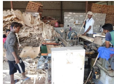
Figure 2: peeling of Wood
