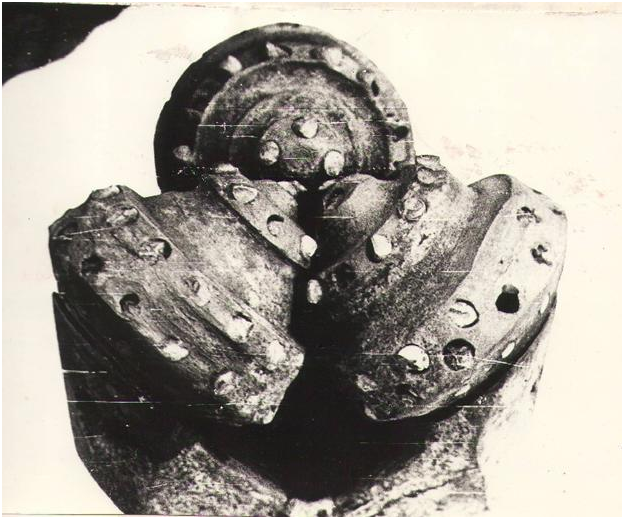
Fig. 2: A characteristic type of destruction of the cutting structure of spent Sh215,9TKZ-TsV-3 bits
