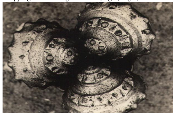
Fig.1: A characteristic type of destruction of the cutting structure of spent Sh215,9K-PV bits
