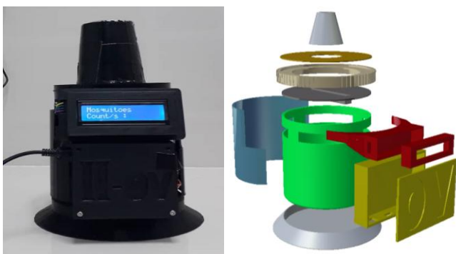
Fig. 7. Prototype D of IoT-based ovitrap system (The height of entrance cone was changed).
