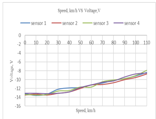
Fig. 11 High Flap Sensors At the Angle 0°
