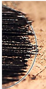
Fig. 4. Optical micrograph of wear scars for mineral oil (magnification 200X)
