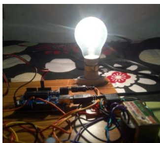
Fig 5 : Light glowing when the attention level is beyond 30
