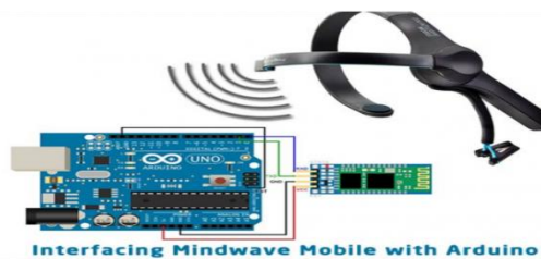
Fig 4 : Interfacing Brain-sense with Arduino UNO
