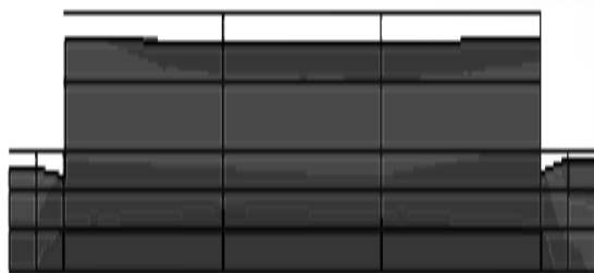
Fig. 4. Deformation state of the base under the influence of own weight (b), weight and hydrostatic pressure of water (c)
