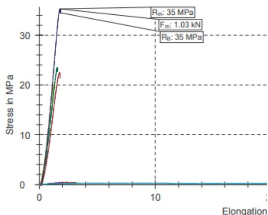
Fig. 7 Tensile strength of PLA- WO3T3 nanocomposite
