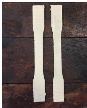
Fig. 4 Tensile specimen fabricated via 3D printing machine following ASTM D638 standard.
