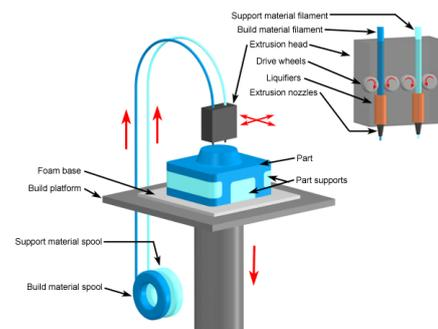
**Fig. 1 3D printing extrusion process [7]**
