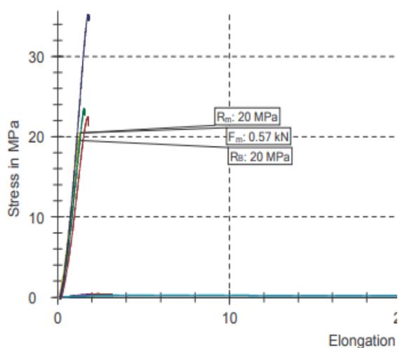
Fig. 6 Tensile strength of Neat PLA
