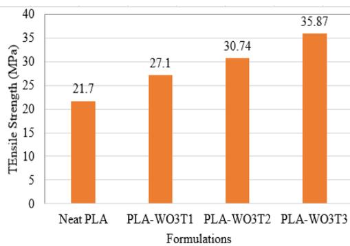
Fig. 5 Tensile strength of Poly Lactic Acid (PLA) – Tungsten Trioxide (WO<sub>3</sub>) Nanocomposites
