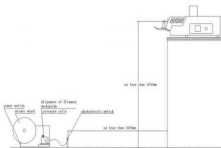
Fig. 3 The alignment of extruder and winder
