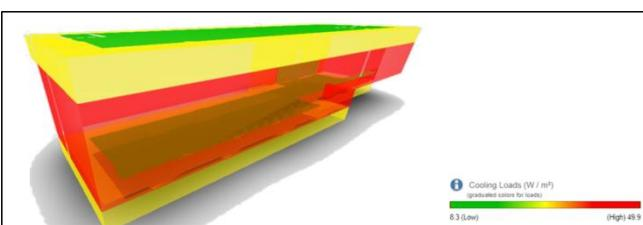
**Fig. 10 Cooling loads for PMU Brickfield.**
