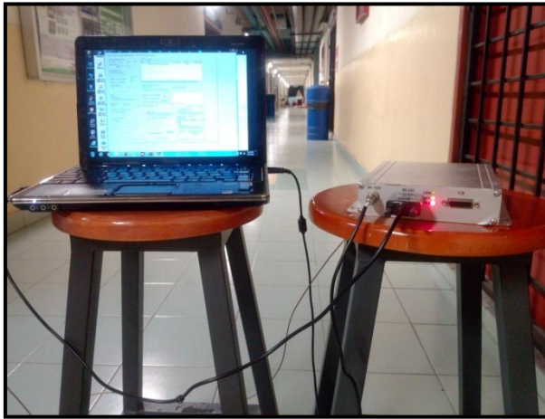
Fig.7 RFID reader connected to the laptop through RS 232
