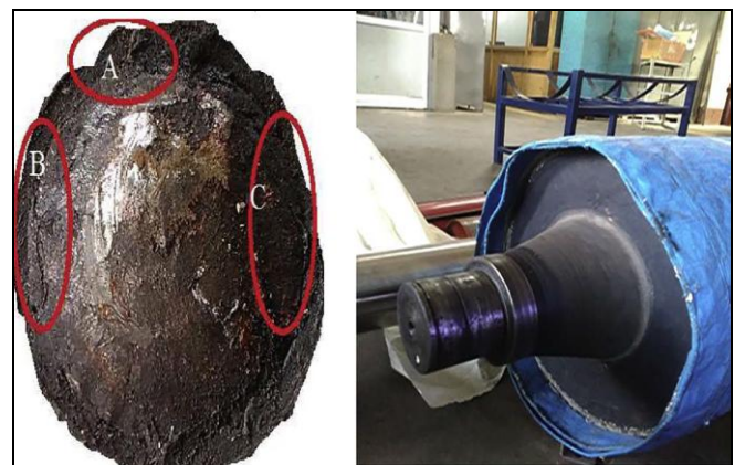
Fig. 2. Failure locations of roller shaft of pad steam machine
