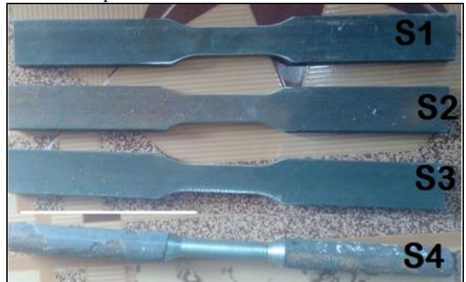
Fig.11 Prepared sample for Tensile test Specimen
