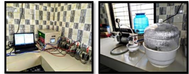
Fig-3: RCPT of concrete samples.
