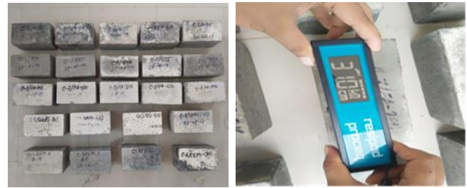
Fig. 2. Samples for ERT of concrete.
