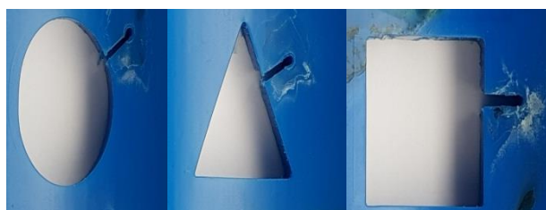
Figure1. The inner face of samples under CO 2 laser cutting using air as assistance gas
