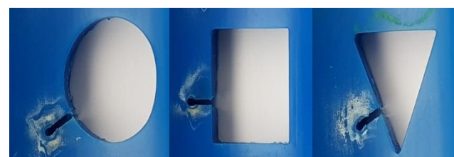
Figure2. The inner face of samples under (CO 2 ) laser cutting using (N 2 ) as assistance gas
