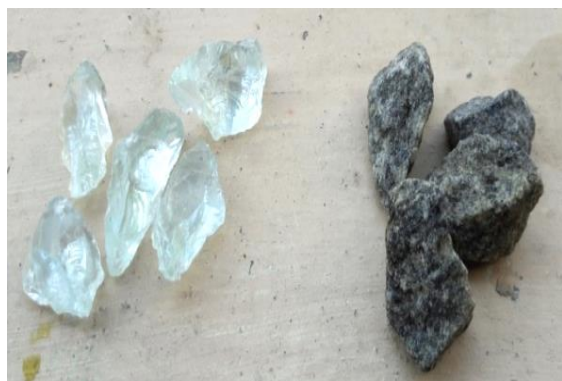
Figure I Recycled Glass Coarse Aggregate sample with Crushed Stone Aggregate
