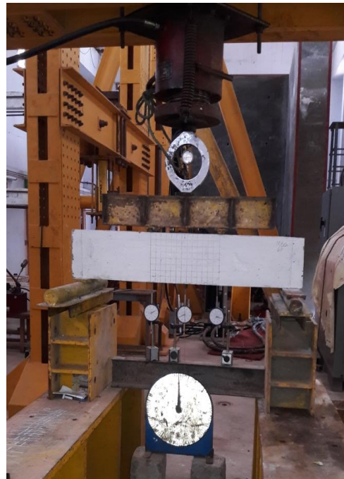
Figure V Flexural Test on Beam Specimen
