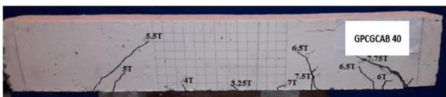
Figure XV Crack Patterns of M 40 GPCGCA Beam
