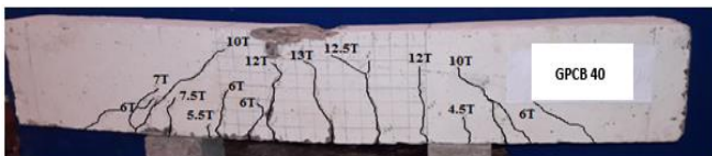
Figure XIV Crack Patterns of M 40 GPC Beam
