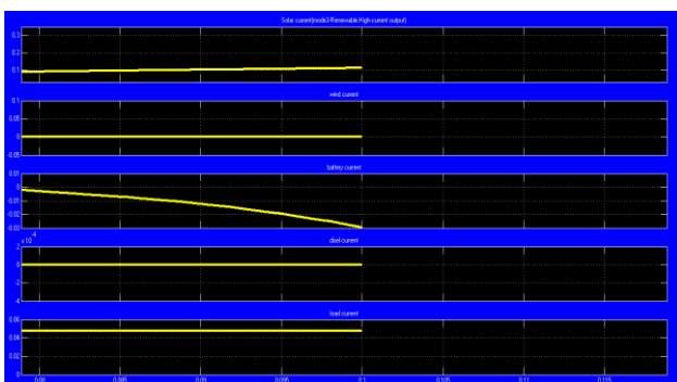
Fig. 15 Mode3 current output waveforms (Renewable high)
