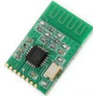
Fig.2 ZigBee Communication Module
