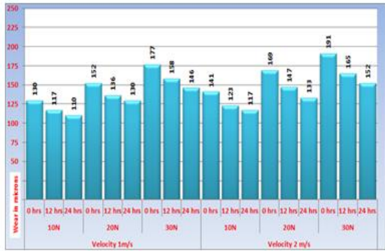
Fig. 10. Wear loss of LM25-10% fly ash composites
