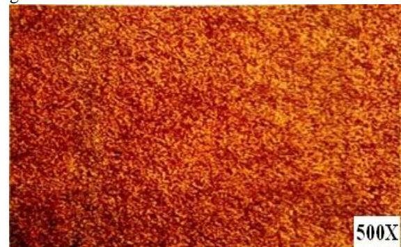
Fig. 4. Microstructure of the LM 25 alloy before deep cryogenic treatment
