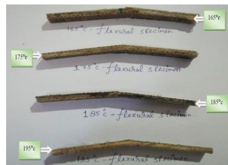
Fig.4. Fractured flexural specimens
