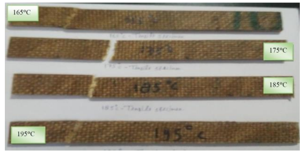
Fig. 2. Fractured tensile specimens
