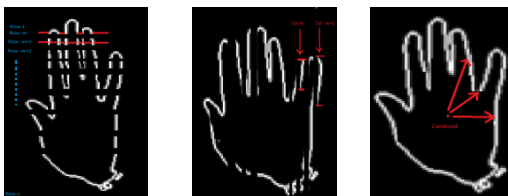
Fig. 3. Proposed region counting across the rows and columns for forming the shape descriptor from the hand shape boundary. Centroid computed for given gesture boundary and the distances taken at different angles
