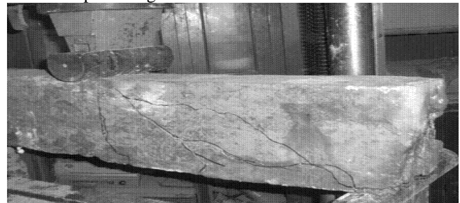
Fig. 6. Typical Failure mode for the four beams
