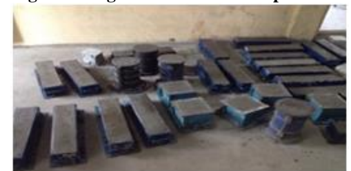
Fig.2 Casting of Cylindrical and Beam Specimens
