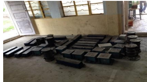
Fig.1 Casting of Concrete Cube Specimens
