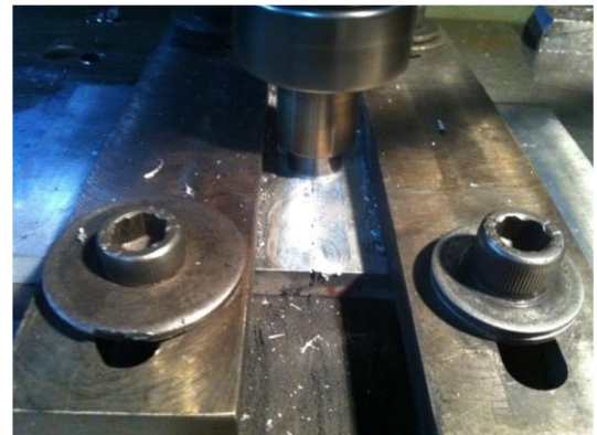
Figure 5 FSP operation with Square Pin Tool Table II: Process Parameters for FSP
