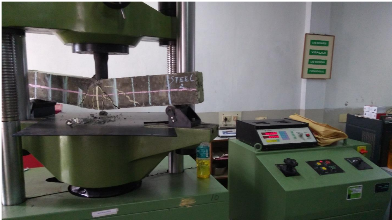
Figure 2- Testing of beam reinforced with steel rebar
