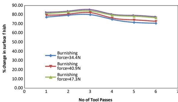
Fig. 6 Percentage of change in surface finish for different number of passes
