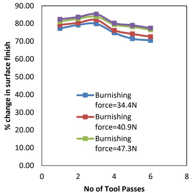
Fig. 4 Percentage of change in surface finish for different number of passes
