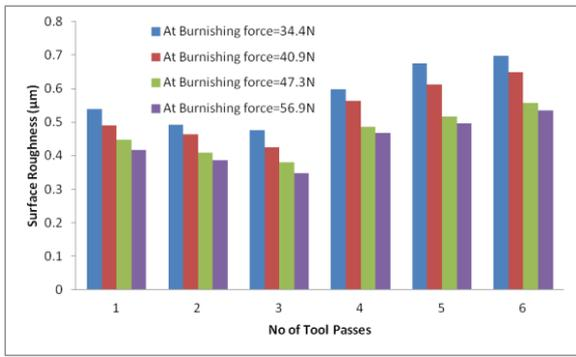
Fig. 5 Variation of surface roughness after burnishing for different number of passes
