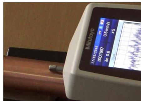
**Fig 2 Surface roughness measurement**
