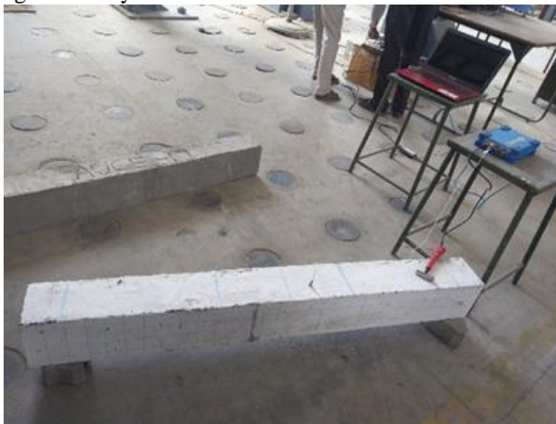
Fig.2. Testing of C&D-Waste Beam using FFT Analyzer
