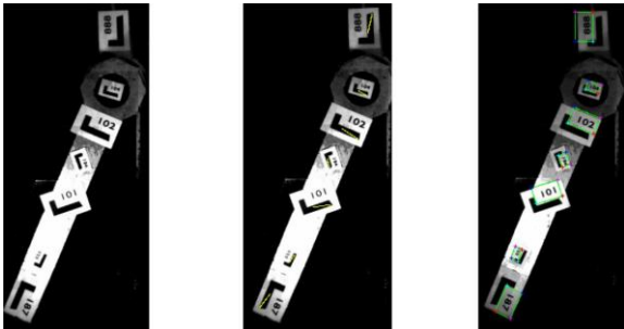
(a) Original image (b) Orientation vectors (c) Text boxes identified Fig. 6: Determination of marker orientation and text bounding box
