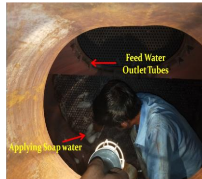
Figure – 7 Soap water test
