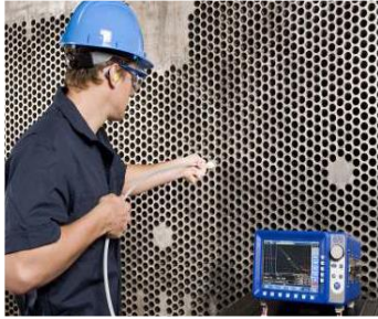
Figure – 5 Eddy Current Test
