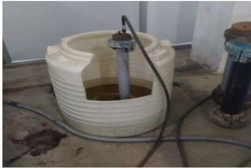
Figure 9 - Bursting Test of PVC Pipe
