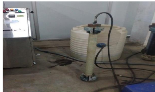
Figure 7 - GFRP Pipe Connected with Pressure Lines for Testing
