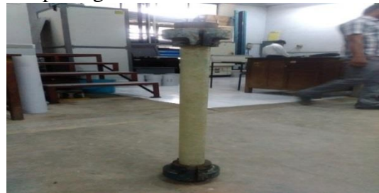
Fig.6 Fixture of GFRP Pipe Before Testing
