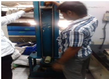
Figure - 4 Impact Test on GFRP Pipe Specimen
