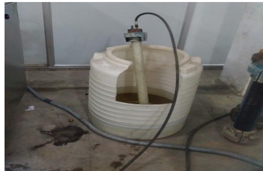
Figure - 8 Bursting Test of GFRP Pipe
