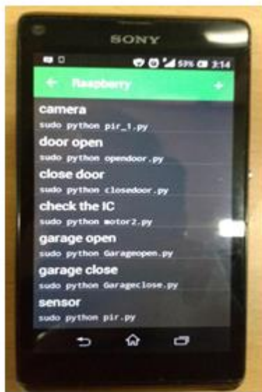
Fig.7 Remotely controlling the Raspbian software from cellular system
