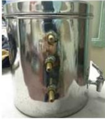
Fig.2 Water level detection using copper bolts
