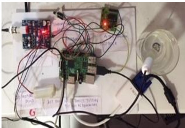
Figure 5 Hardware setup of water quality testing system.
